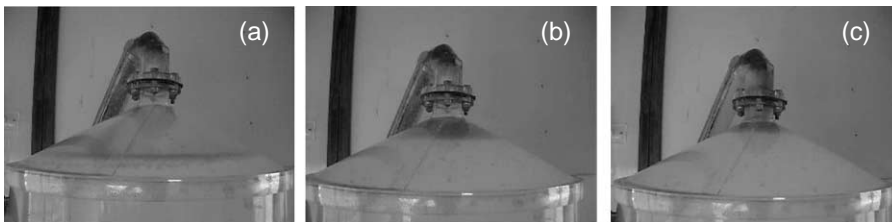
Figure 2 Automatic discharge of accumulated scum through the top outlet of the DOF separator: (a) water level rises as the magnetic valve is closed; (b) water level rises to the outlet; (c) scum being discharged through the outlet
